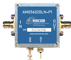
AMCOM AM056020LN-P1 is a broadband Low Noise Amplifier module. It is designed for general purpose applications. It operates from 500 MHz to 6000 MHz with mid-band Noise Figure of 2 dB and small signal gain of 20 dB.
