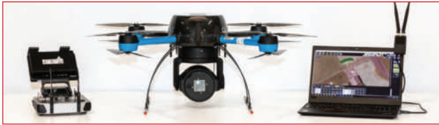
▲ Fig. 4 From left to right: drone manual controller (used only for take-off and landing); drone equipped with a RF payload; base station.
