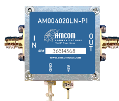
AMCOM AM004020LN-P1 is a broadband Low Noise Amplifier module. It is designed for general purpose applications. It operates from 20 MHz to 4000 MHz with Noise Figure of 2 dB and small signal gain of 24 dB.
