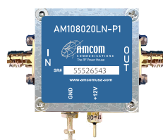
AMCOM AM108020LN-P1 is a broadband Low Noise Amplifier module. It is designed for general purpose applications. It operates from 1 GHz to 8 GHz with mid-band Noise Figure of 2 dB and small signal gain of 22 dB.
